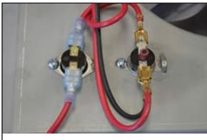
Thermal protection with automatic reset that will shut the heating element off in case of overheating.
