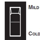
The **SPEED SELECTOR** switch is used to control the fan speed (ventilation). Even if there is no call for heat, the ventilation can be controlled by the thermostat; the fan speed is determined by this switch.
