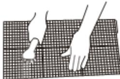
3. Install filter: after the filter is cleaned and dried, reinstall it well.
